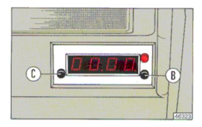
The chronometer can display up to 9h59min, so it may be used to time a trip.
