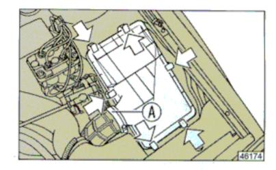
Remove the housing cover. Clean or replace filter element B.
