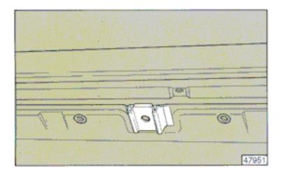
If the jack is placed at any other position, it may be dangerous to lift the car and damage to the lower body moulding can occur.
