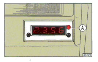
The current time can be displayed during chronometer operation by pressing button A.
