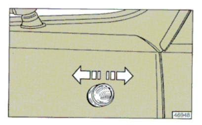
Move the lens slightly forward or towards the rear of the car. Rotate gently to remove the bulb holder. Remove and replace the capless 5W bulb. Aligning the headlight beams from inside the car (if fitted)
