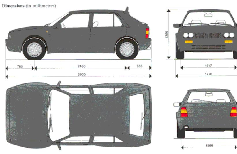
Luggage compartment volume (VDA standards): 200 dm<sup>3</sup>. Cargo area (rear seat folded down) (VDA standards): 940 dm<sup>3</sup>. Heights indicated for unladen cars.
