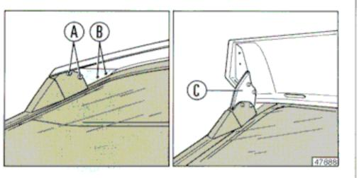
If you wish to raise the spoiler, unscrew the four screws A (2 on each side), and reattach the spoiler at holes B using the same screws.
