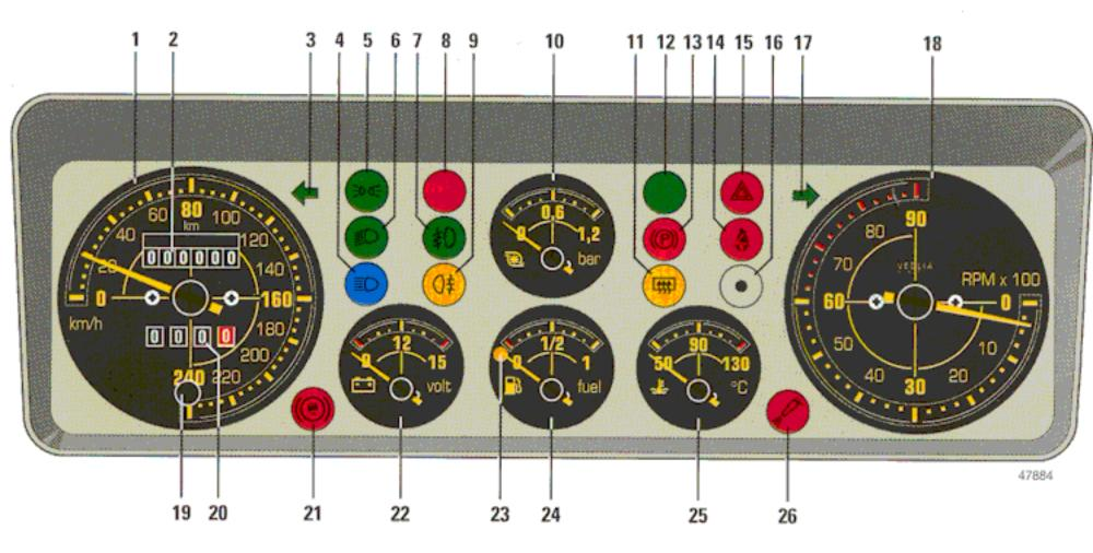
\* In the "kat" version indicator 26 signals maximum turbocharger capacity (see p. 10).
