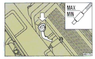
When topping up or changing the oil, run the engine for a couple of seconds then wait a few minutes before rechecking the level.
