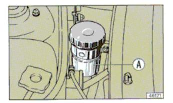
Use only DOT 4 class brake fluid for topping up. Tutela DOT 4, used when the car is manufactured, is recommended. Fluids with different characteristics will damage the rubber seals.
