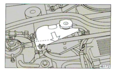
Top up or change the coolant using a 50-50 mixture of antifreeze and distilled water. **FIAT Paraflu**<sup>11</sup> is the recommended antifreeze. When the engine is hot never remove the expansion tank cap to prevent being scaled.
