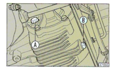
When the level is near or below MIN, top up through the dipstick housing until reaching MAX.
