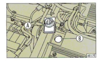
The oil level should always be between the MIN and MAX marks on the dipstick. When the level drops below the MIN mark add oil through filler hole B after removing cap A until reaching the MAX mark on the dipstick. Never exceed the MAX mark. The difference between MIN and MAX corresponds to about 1 litre of oil.
