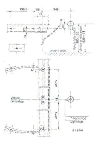
The tow hitch installer is required to fasten a plate at the same level as the hitch bearing the following information: MAXIMUM LOAD AT THE COUPLING 70 kg.
